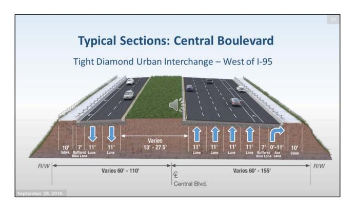
West of the interchange, Central Boulevard northbound would be expanded to two 11-foot travel lanes, two 11-foot auxiliary lanes, a 7-foot buffered bicycle lane, an 11-foot auxiliary lane, and a 10-foot sidewalk. In the southbound direction would be two 11-foot travel lanes, a 7-foot buffered bicycle lane, and a 10-foot sidewalk.
