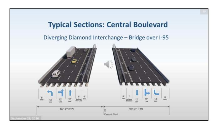
The DDI alternative would involve replacing the existing Central Boulevard bridge over I-95 with a pair of bridges. On each would be three lanes for through and turning traffic, an 8-foot shoulder next to the outer edge, and a 7-foot buffered bicycle lane and 6-foot covered sidewalk next to the inner edge.
