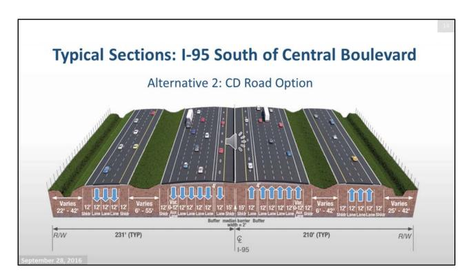
South of Central Boulevard, a CD road would be constructed on either side of I-95. It would include three 12-foot lanes and two 12-foot shoulders.
