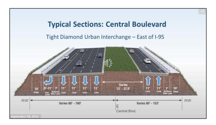
East of the interchange, the reverse would occur: Central Boulevard southbound would be expanded to two 11-foot travel lanes, two 11-foot auxiliary lanes, a 7-foot buffered bicycle lane, an 11-foot auxiliary lane, and a 10-foot sidewalk. In the northbound direction would be two 11-foot travel lanes, a 7-foot buffered bicycle lane, and a 10-foot sidewalk.
