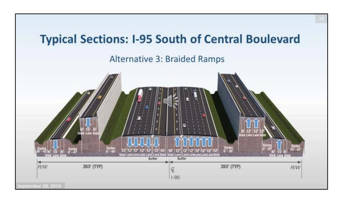
South of Central Boulevard, the Central Boulevard off-ramp would be two 12-foot lanes with 8-foot and 12-foot shoulders. The Military Trail off-ramp would be one 15-foot lane with 6-foot shoulders on both sides. The on-ramps would be one 15-foot lane with 6-foot shoulders on both sides.
