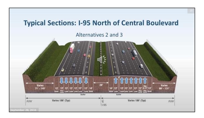
North of Central Boulevard, in addition to the existing travel lanes, the I-95 section would include two 12-foot auxiliary lanes in the northbound direction, one 12-foot auxiliary lane in the southbound direction, 12-foot outside shoulders, and 14-foot inside shoulders.
